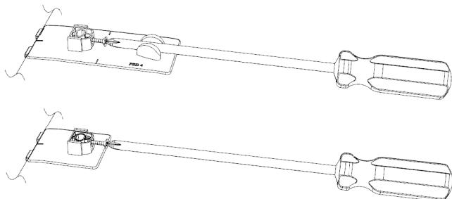
11. Insert a screw into each base a few turns. The tip of the screw should not protrude into the hole where the retaining pin will be installed later.
