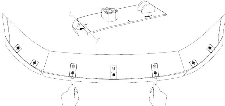
12. Peel and fold the anti-abrasion film pads in half over the hood edge between the fingers on each of the large pedestals in the locations shown.
