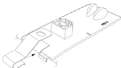
13. Push metal mounting brackets over the hood edge aligned with the anti-abrasion pads. Ensure the bracket is fully seated over the hood edge and the hole in the bracket is aligned with the hole in the pedestal.
