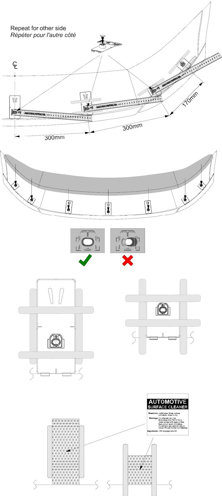
6. Dry fit the pedestals using tape strips supplied or masking tape to temporarily hold them in position. The positions of the pedestals are shown in the illustrations. Use the center line on the leading edge of the pedestals for accurate measuring. The pedestals install perpendicular to the hood edge.
