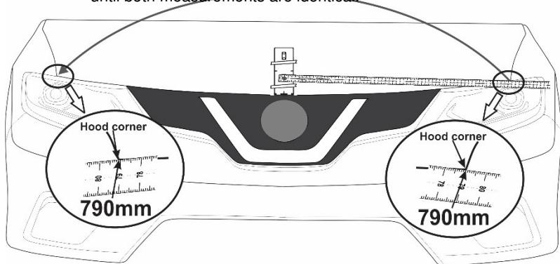
\* Tape measure is always located below the measuring point\*
