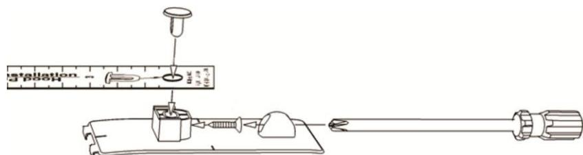
**Locate center pedestal using installation tape measure and/or the supplied centering template.**
