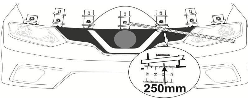
4. Starting at the outer most locations dry fit the remaining pedestals using masking tape or re-usable tape strips supplied to temporarily hold them in position.
