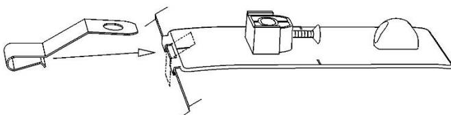
11. Push metal mounting brackets over the hood edge aligned with the anti-abrasion pads installed previously. Ensure each bracket is fully engaged over the hood edge and the hole in the bracket is aligned with the hole in the pedestal. In the locations shown.
