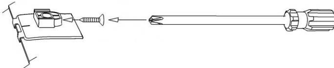
9. Start a screw into each pedestal a few turns. The tip of the screw must not protrude into the hole where the attachment pin will later install.
