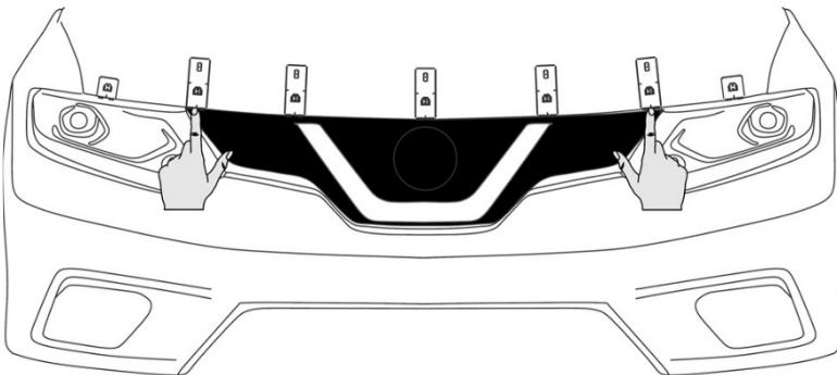
10. Peel and fold the anti-abrasion pads in half over the hood edge between the fingers on the pedestals. In the locations shown.
