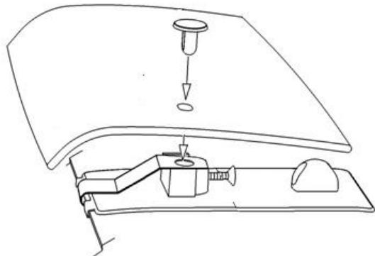
10. Place the protector on the pedestals and, starting at the center location, install a pin through the protector and into the pedestal. Maintain slight pressure on the pin, to ensure proper seating of the components, while simultaneously tightening the screw on each of the adhesive pedestals.
