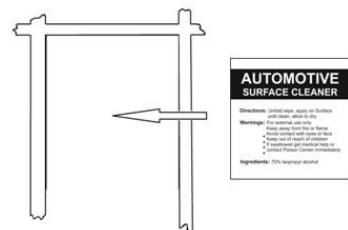
5. Remove the pedestals and thoroughly clean the outlined area with the Automotive surface cleaner. Wipe dry with a clean cloth or paper towel. This will insure all wax, finger prints and oils are removed from the hood surface in the bonding area.
