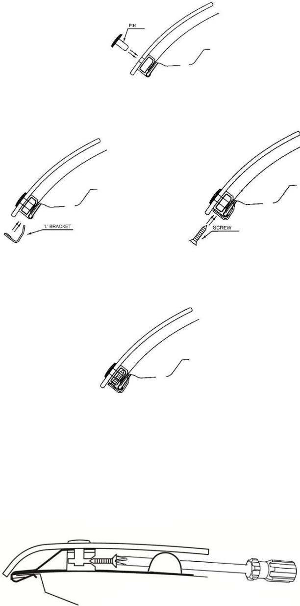
13. Insert a pin through the protector into each of the clip bodies.
