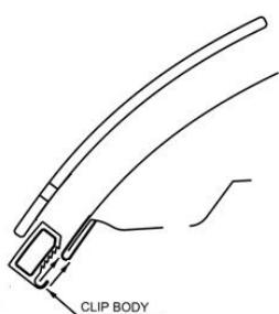
12. Place a clip body over each of the abrasion pads on the edge of the hood.
