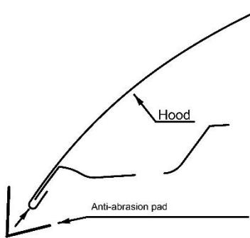
11. Peel and fold the six (6) abrasion pads in half over the hood edge aligned with the outer holes of the protector in the area above the headlights.
