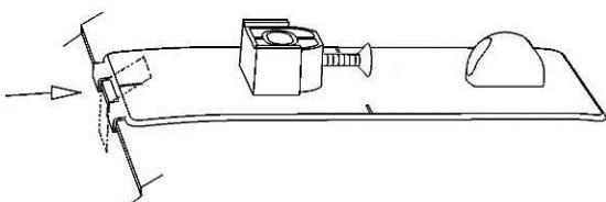
8. Peel and fold an anti-abrasion pad in half over the hood edge between the fingers on each pedestal.
