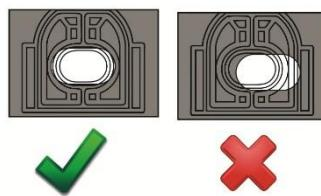
1. The positions of the other pedestals are shown in the illustration. Use the center mark on the leading edge of the pedestals for accurate measuring. The fingers incorporated on the leading edge of the pedestal will help ensure the correct position relative to the hood edge. When correctly positioned the fingers should contact the leading edge of the hood. Temporarily locate the pedestals using repositionable tape strips or masking tape.
