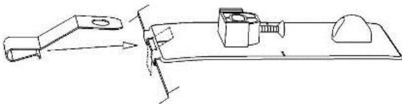
9. Push metal mounting brackets over the hood edge aligned with the anti-abrasion pads installed previously. Ensure each bracket is fully engaged over the hood edge and the hole in the bracket is aligned with the hole in the pedestal.
