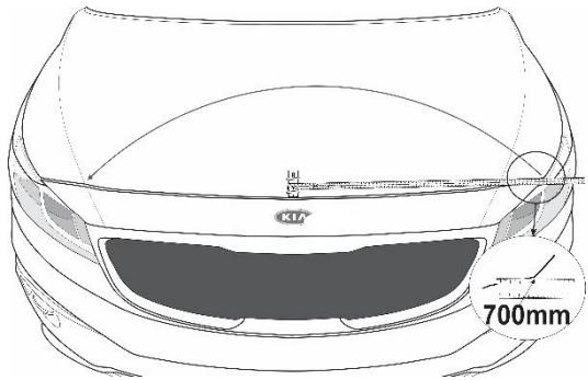
\* Tape measure is always located below the measuring point.
