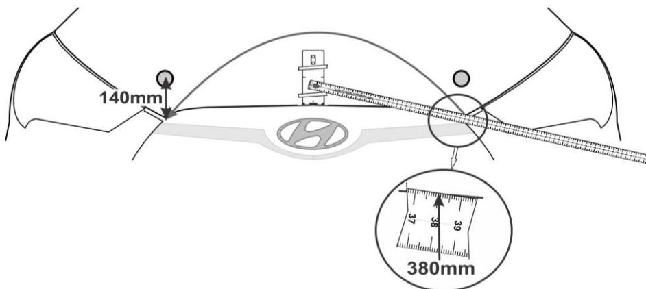
**Locate bumpons using installation tape.**
