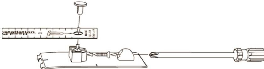
**Locate centre pedestal using installation tape.**
