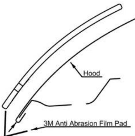
11. Peel and fold the four (4) large anti-abrasion film pads in half over the hood edge aligned with the outer holes of the deflector in the area above the headlights.
