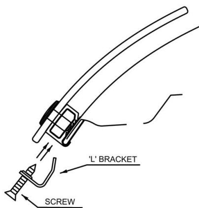
14. Insert a #6 x 5/8" screw through an 'L'- bracket and into the clip body.
