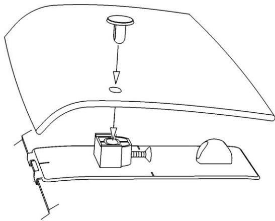
9. Place the deflector on the pedestals and drop a pin through the deflector and into the pedestal.
