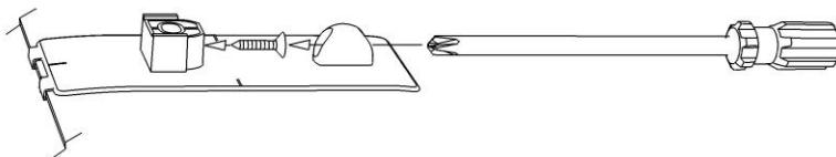
8. Start a #6 x 5/8 flat head screw into each pedestal a few turns. The tip of the screw must not protrude into the hole where the attachment pin will install later.
