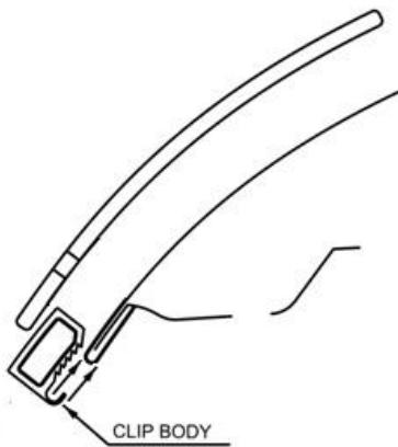
12. Place a clip body over each of the anti-abrasion film pads on the edge of the hood.
