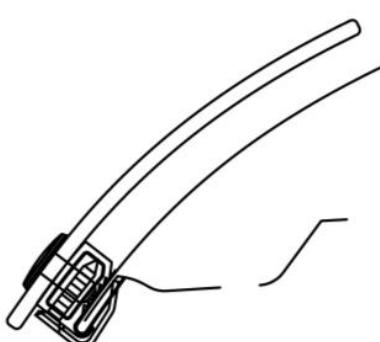
15. Make sure all the components are well seated together and then tighten the screws into the clip bodies.
