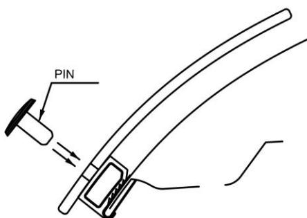
13. Insert a pin through the protector into each of the clip bodies.
