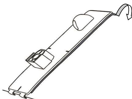
6. Remove the pedestals and thoroughly clean the outlined area with the alcohol wiping pad. This will insure all wax, finger prints and oils are removed from the hood surface in the bonding area.
