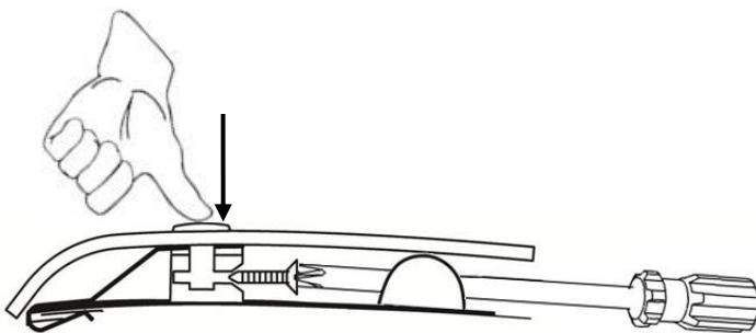
10. Maintain slight pressure on the pin, to ensure proper seating of the components, while simultaneously tightening the screw. Repeat for remaining pedestal locations.
