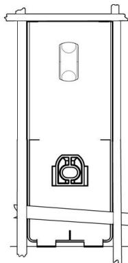
4. Install the two (2) bumpons as shown. **Attention:** **Bumpons must be installed on the hood, not on the deflector.** If the bumpons are installed on the deflector, they may wear through the paint.
