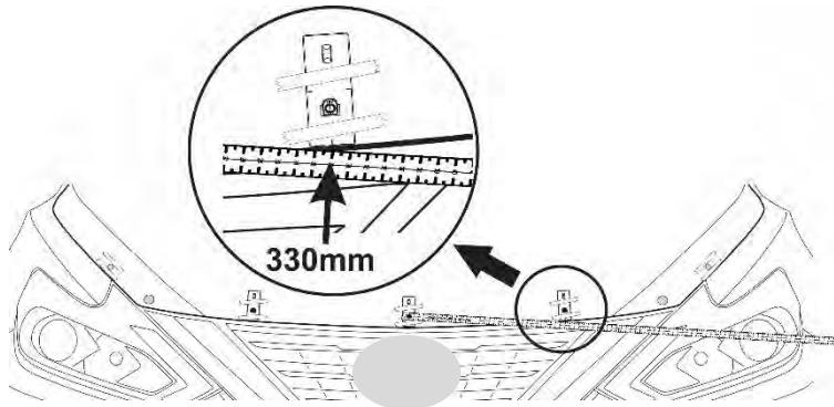
5. Using the repositionable tape strips, temporarily attach the two (2) large adhesive pedestals at the location indicated in the illustration.
