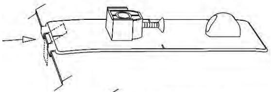
11. Peel and fold an anti-abrasion pad in half over the hood edge between the fingers on each pedestal.
