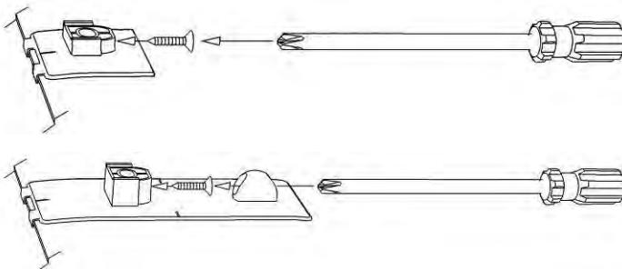
8. Remove the pedestals and thoroughly clean the outlined area with the alcohol wiping pad. Wipe dry with a clean cloth or paper towel. This will insure all wax, finger prints and oils are removed from the hood surface in the bonding area.
