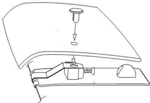
13. Place the protector on the pedestals and, starting at the center location, install a pin through the protector and into the pedestal. Maintain slight pressure on the pin to ensure proper seating of the components, while simultaneously tightening the screw a few turns. Repeat for remaining pedestal locations.
