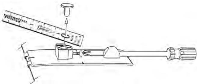
6. Remove the hood protector installation tape measure. Place the hood protector on the pedestals to confirm proper positioning. Ensure the holes in the protector align with those in the pedestals. If necessary, reposition the pedestals so all attachment positions are correct and the protector is well centered.
