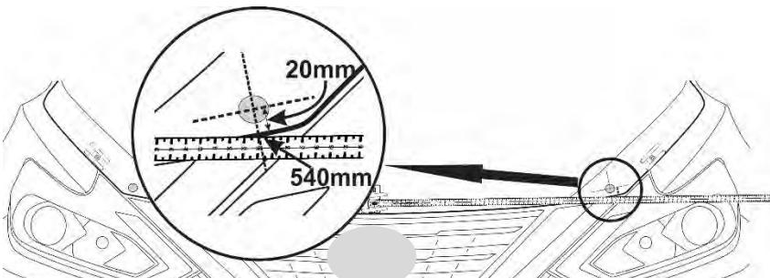
1. Assemble the installation tape measure as shown in the illustration.
