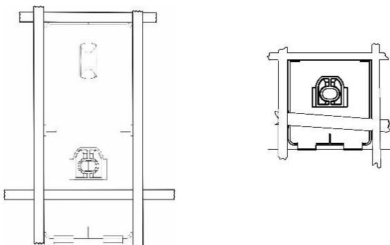
7. Remove the hood protector, and outline the perimeter of the pedestals with masking tape or the re-usable tape strips supplied to help final installation.
