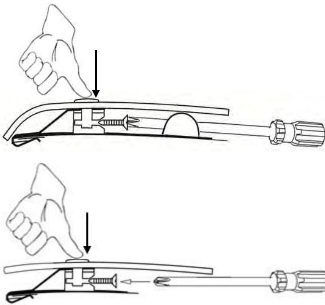
14. Starting at the center location tighten all the screws that were loosely installed in step 13. To ensure proper seating of the components, maintain slight pressure on the pin while simultaneously tightening the screw.
