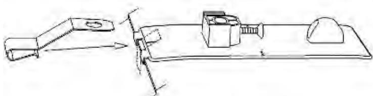
12. Push metal mounting brackets over the hood edge aligned with the anti-abrasion pads installed previously. Ensure each bracket is fully engaged over the hood edge and the hole in the bracket is aligned with the hole in the pedestal.
