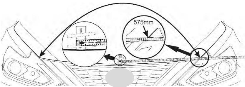
\* Tape measure is always located below the measuring point\*
