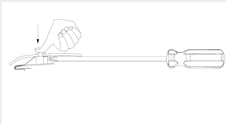
10 Maintain slight pressure on the pin to ensure proper seating of the components, while simultaneously tightening the screw a few turns. Repeat for remaining pedestal locations.
