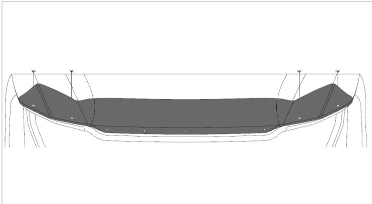
9 Place the protector on the pedestals and starting at the center position, install a pin through the protector and into the pedestal.
