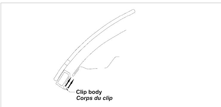
12 Place a clip body over the anti-abrasion film pad on the edge of the hood.
