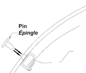
13 Insert a pin through the protector and into the clip body.
