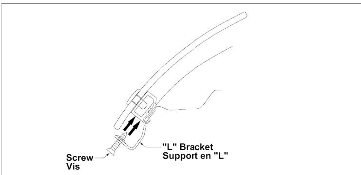
14 Place an "L" bracket over the hood edge and against the clip body. Installer la vis et le support en "L"
