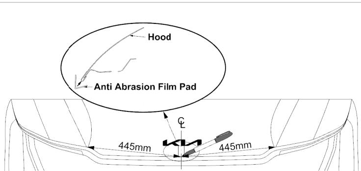
1. Use measurements to estimate centre of the hood and wrap masking tape over the hood edge.
