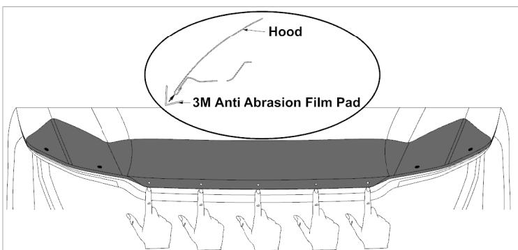
11 Centre the protector by equalizing the overhang on each side of the protector.
