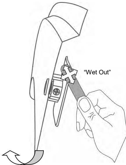
8. Once the visor is in place, press down **hard** along the entire flange area to make sure that the adhesive tape is fully adhered to the vehicle.
