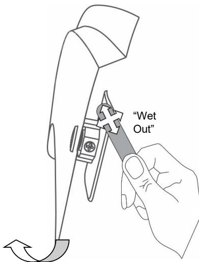
7. Gently lift visor away from door frame so the pull tab on the adhesive pedestal is accessible. Pull the red backing from the pedestal and firmly press the visor onto the door frame. Using the wooden "wet-out" stick supplied, reach under the visor to apply pressure to the surface of the adhesive pedestal. This will make sure there is maximum contact between the adhesive tape and door frame.
