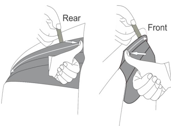
**9** Confirm visor placement. Press visor into place at the mirror base.
