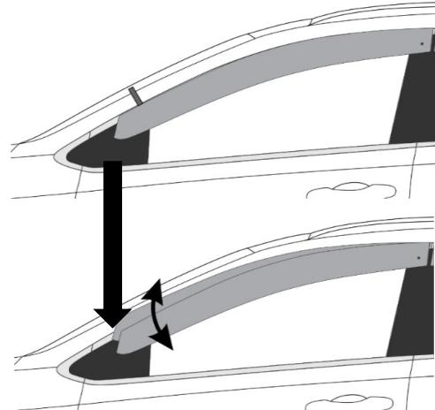
**8** Pivot the visor into position. The visor should index with the transition from the mirror base and door flange with equal amount of trim visible, front and back. Peel a small quantity of the two-sided tape protective backing at the mirror base end so there is a small pull-tab. Do not press the visor into place at this stage.
