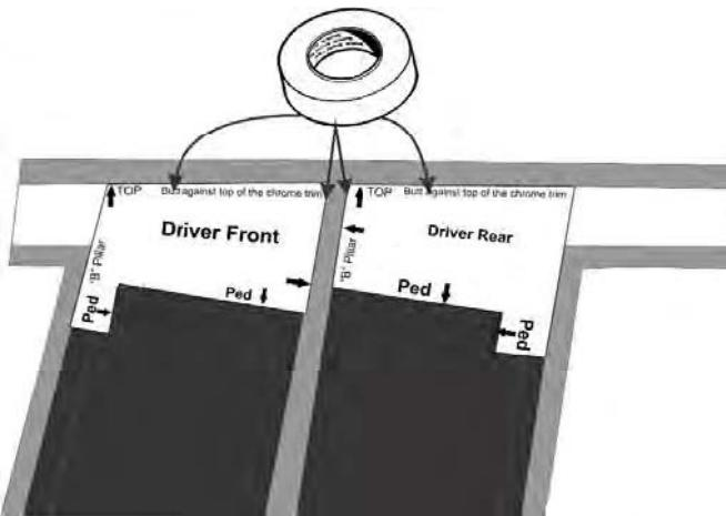
There are 2 templates. Each is labeled for its position. The templates will guide in the positioning of the mounting pedestals. As noted on the template, each is intended for a specific location.
