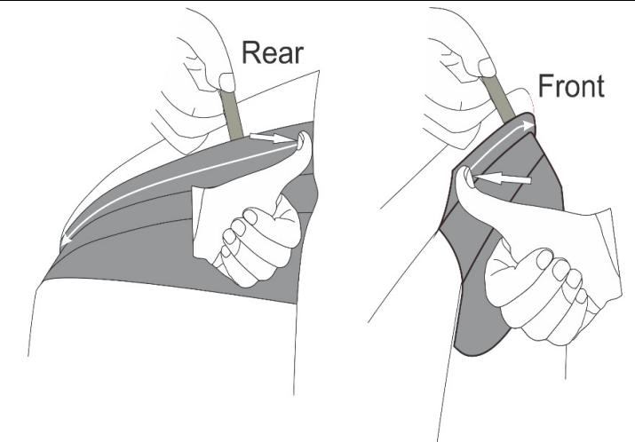
10 Simultaneously peel backing and softly press the middle of the flange into place while ensuring the placement remains correct and the amount of chrome is consistent along the door frame. Once all the protective backing has been removed, press hard along the whole length to ensure the tape is properly adhered.
