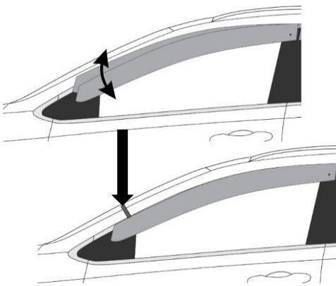
**7** Mount the visors one at a time, starting with the driver front.
