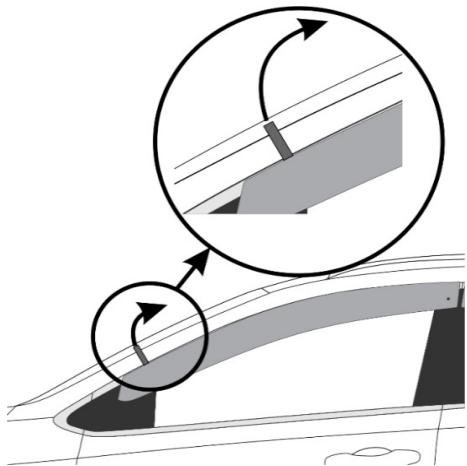
9 Confirm visor placement. Press visor into place at the mirror base.
