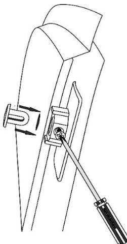
**7** Mount the visors one at a time, starting with the driver front. Place a screw in the screw hole in the mounting pedestal. Only turn it enough to keep it in place. Push a pin through the visor and into the mounting pedestal as shown. Turn the screw in a few turns but do not tighten in place. This will hold one end of the visor while you align the other.
