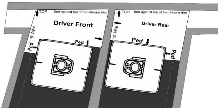
Note the position of the mounting pedestals. The screw hole in the raised portion of the pedestal faces the door opening or "B" pillar. On the front door it faces rearward. On the rear door it faces forward.
