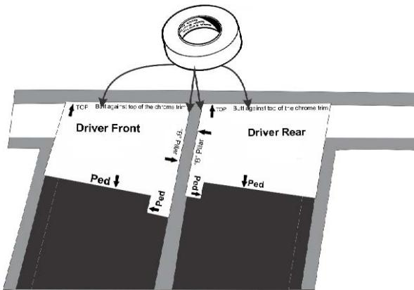
1 Locate template sheet in the kit. Cut out the templates.
