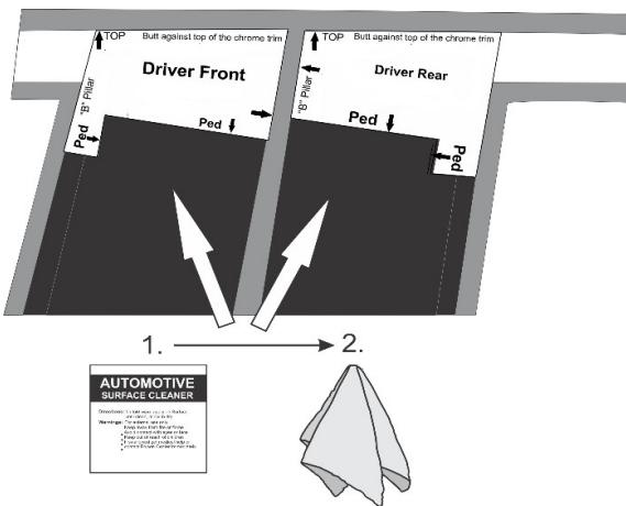
Remove the pedestal and thoroughly clean the area with the surface cleaner. Wipe dry with a clean cloth or paper towel. This will insure all wax, finger prints and oils are removed from the hood surface in the bonding area.
