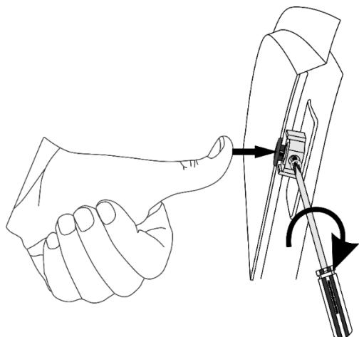
11 Ensure the pin is properly seated and tighten the screw into the mounting pedestal on each visor. It will be necessary to open the front doors to do this. Take care to not overtighten the screw.
