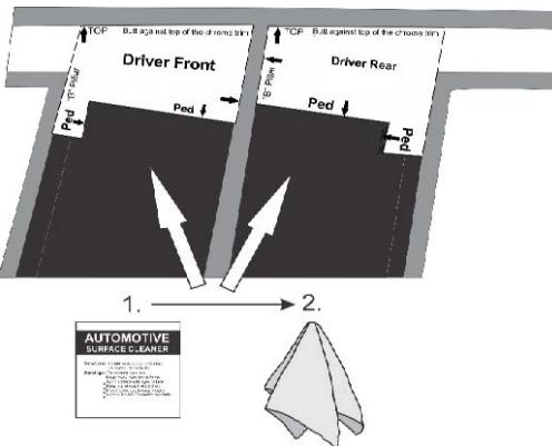
3 Note the position of the mounting pedestals. The screw hole in the raised portion of the pedestal faces the door opening or "B" pillar. On the front door it faces rearward. On the rear door it faces forward. **\*Do not peel backing and stick pedestal down at this point.\*\***
