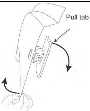
9 Gently lift visor away from door frame so the pull tab on the adhesive pedestal is accessible. Pull the red backing from the pedestal and firmly press the visor onto the door frame.
