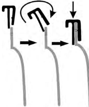
1 Using the method illustrated, snap two (2) clips on each visor. Note orientation of the clip.
