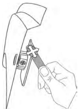
11 Using the wooden "wet-out" stick supplied, reach under the visor to apply pressure to the surface of the adhesive pedestal. This will make sure there is maximum contact between the adhesive tape and door frame.
