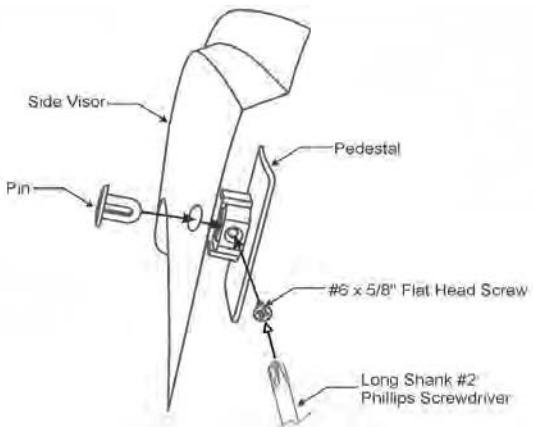
2 Insert a pin through the hole in the side visor and into the adhesive backed pedestal. Maintain slight pressure on the pin, to ensure proper seating of the components, while simultaneously tightening the screw.
