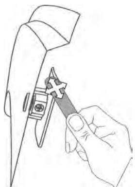
11 Using the wooden "wet-out" stick supplied, reach under the visor to apply pressure to the surface of the adhesive pedestal. This will make sure there is maximum contact between the adhesive tape and door frame.
