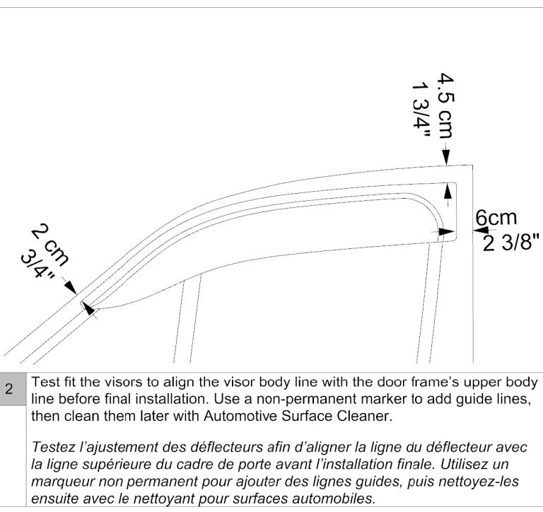
**2** Test fit the visors to align the visor body line with the door frame's upper body line before final installation. Use a non-permanent marker to add guide lines, then clean them later with Automotive Surface Cleaner.
