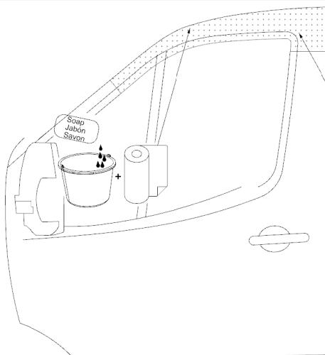
**1** Clean the mounting areas aggressively with alcohol wiping pad and dry with a clean cloth or paper towel to remove any finger prints, oils or waxes that may be on the surface.
