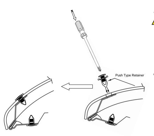
14. Place the hood protector on the hood resting on the four (4) metal brackets; align the 4 center holes in the protector with the holes in the metal brackets. Insert a "push type retainer" through the hole in the protector, and into the bracket. Ensure the protector is well seated against the surface of the metal bracket, and push the center pin of the retainer assembly to lock it into place.
