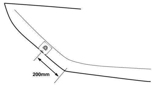
7. The positions of the pedestals are shown in **illustration**. Use the center mark on the leading edge of the pedestal for accurate measuring. The fingers incorporated on the leading edge of the pedestal will help ensure the correct position relative to the hood edge. When correctly positioned the fingers should contact the leading edge of the hood.
